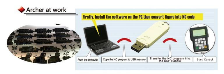
Through USB Port! Input and output the NC program simply.
